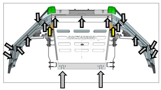
6.1Using below bolt kits: Install the Skid Plates into position, the bulbar has nutserts fitted to the bar allowing a easy fitment,
