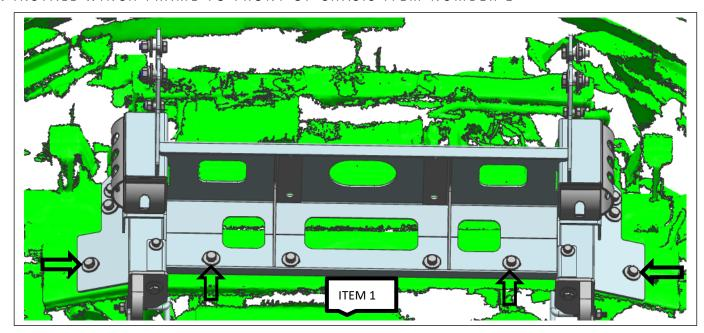
Use below bolt kits: These are mounted into existing vehicle mounting points (Only finger Tighten at this stage)
