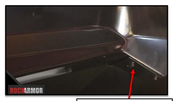
Tighten all bolts once Bash plates are mounted and correctly secured in place
