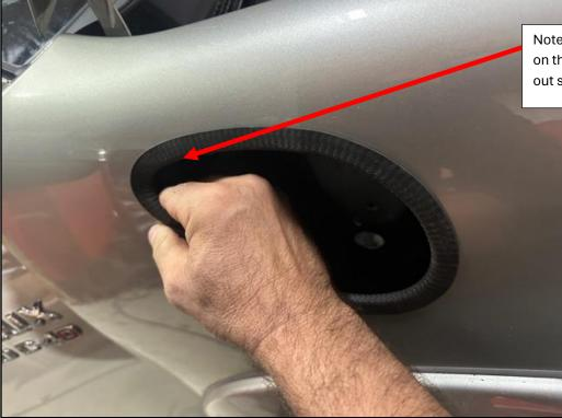
Note: Install the Pinch Weld on the surrounds of the cut out section, cut to size.
