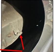
Note: Mounting Bracket/Plate to be used as a support mount for the snorkel, install to the provided mounting plate. Connecting the snorkel to the mounting bracket
