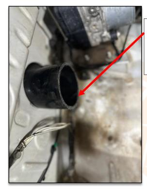
Note: 75mm (3" Inch) Silicon Pipe will be fed though the factory cut so it connects directly to the airbox
