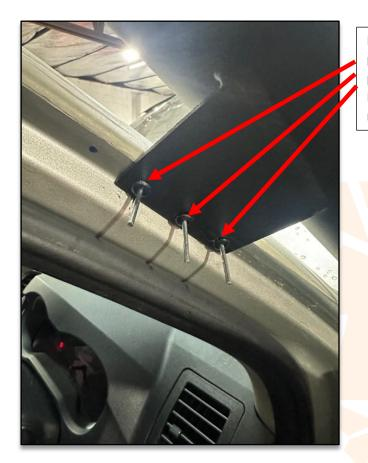
Note: Once the Snorkel sit comfortably through the quarter panel and place into the airbox, then mount the mounting plate from the snorkel to the Drivers side upright support. Mark the 3 holes, drill, apply a bead of Silicone and then rivet the snorkel into the drilled holes
