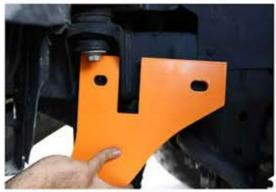
\*Place the Passenger side Recovery point in place like pictured against the 2 holes. This step will 1 person to hold the recovery point with another person to feed through the (black nut with extended wire) through the back hole.
