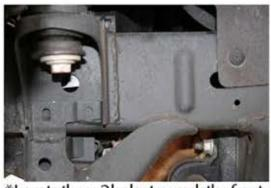
\*Locate these 2 holes towards the front of the chassis rail.
