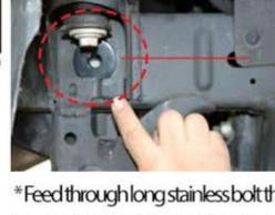
Feed the (black nut with extended wire), from the back hole through to the left hole so it sitting behind the black spacer.
