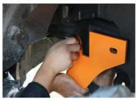
\*Feed through long stainless bolt through the left hole the black nut with the extended wire) WILL capture the long Stainless bolt.
