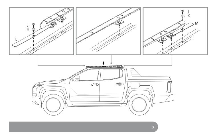
Install the stud plates to the Ridge Mount assemblies.
