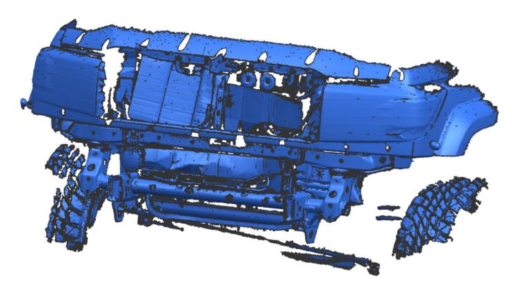
Remove front factory bumper (Take care when unclipping any wiring harnesses)
